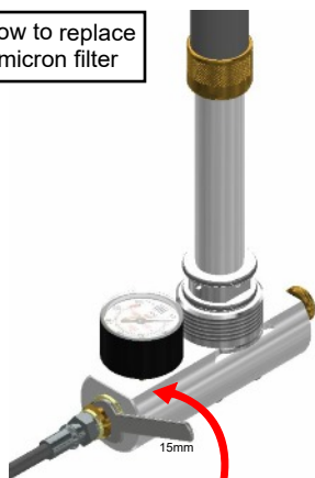
C1. Remove hose end adapter with 15mm spanner
